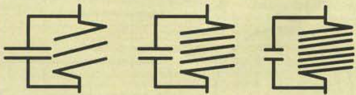
Fig. 3— Different combinations of inductance and capacitance vary the resonant frequency of the tuned circuit and the length of the straight element that will be needed for the next band segment.
